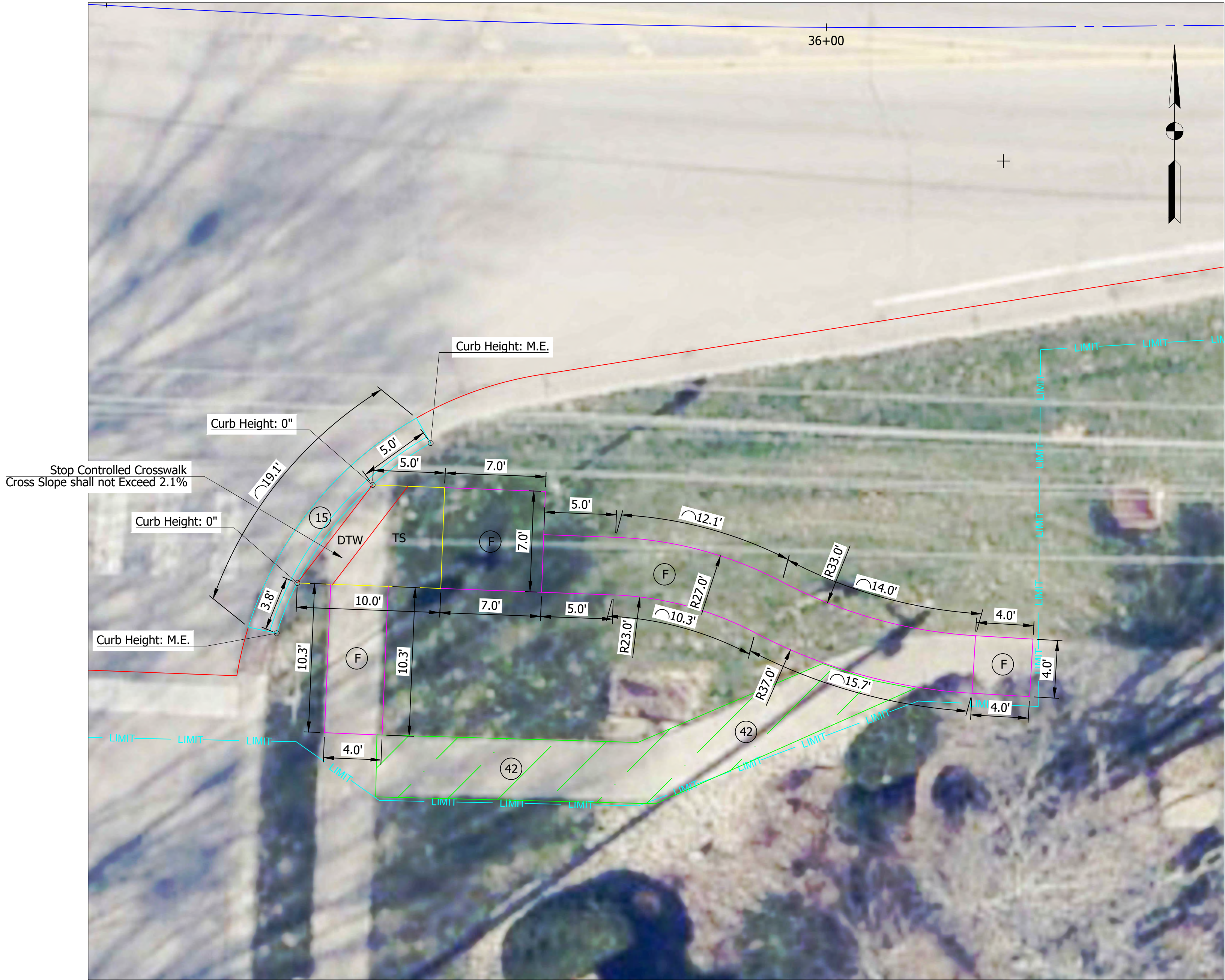
CURB RAMP DETAILS SE CORNER ROGERS ROAD AND THE STANDS DRIVE Scale: 1"=5'
