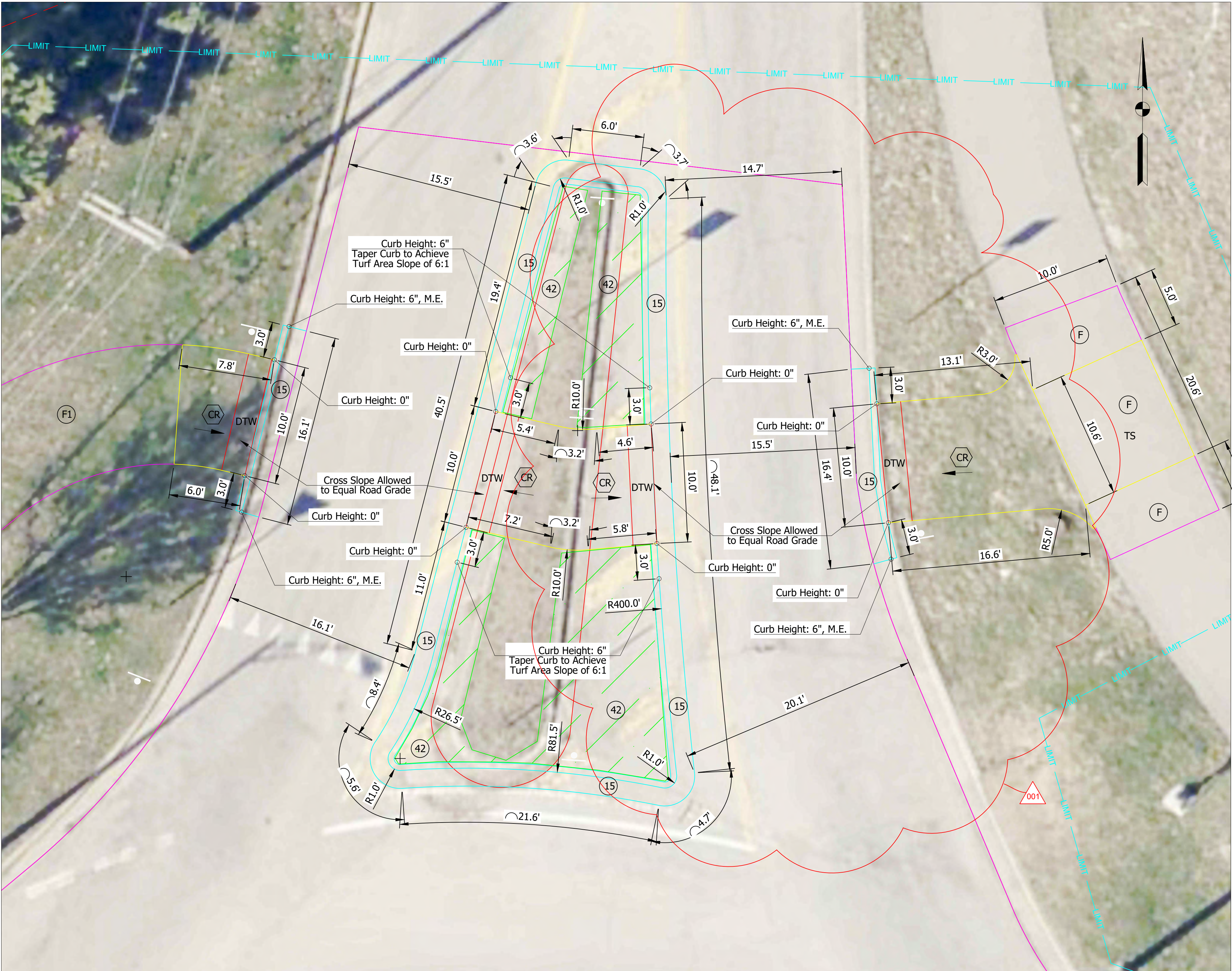
CURB RAMP DETAILS NORTH SIDE WINSLOW ROAD AND HIGH STREET Scale: 1"=5'
